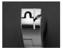
Loop closing plier. For bending of stop loops and ideal for Adams clasps.
