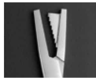
Closing loop plier. Different loops in only one plier.
